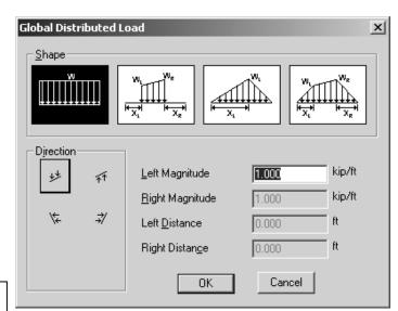
Multiframe will automatically generate a grouping called a Load Case named <u>Load Case 1</u> when a load is created. All additional loads will be added to this load case unless a new load case is defined (Add case under the Case menu).
