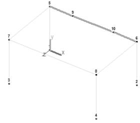
• In order to model a beam end as simply supported, you must release the restraint preventing rotation about the x-x axis of the beam. The pinned ends menu is useful for segments or subdivided members.
